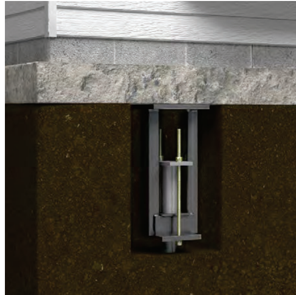
Figure 2.47 Concentric pier installation
